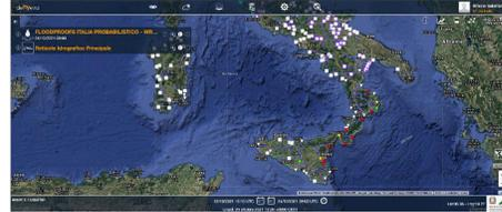
**Figure 30.** OCTOBER 24 at 09 UTC: FloodPROOFS forecast (WRF input) - Expected exceedances: in addition to the sections in Calabria, there are sections in the provinces of Catania and Messina that turn red due to high discharge forecast.
