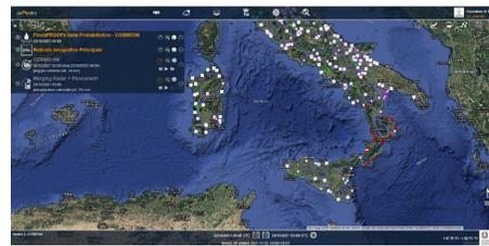
**Figure 27.** OCTOBER 23 at 09 UTC: FloodPROOFS forecast (COSMO 5M input), when the forecast discharge exceed the maximum threshold the marker of the section turn red.
