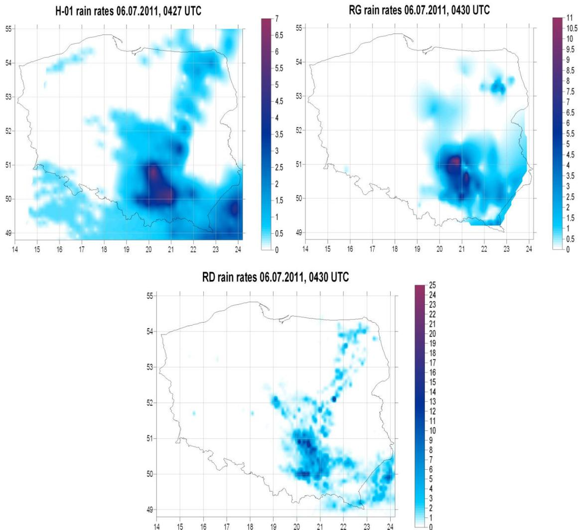
Fig.3 PR-OBS-1 at 0427 UTC on the 6<sup>th</sup> of July 2011 (left panel), 10 minute precipitation interpolated from RG data at 0430 UTC (right panel) and 10 minute precipitation derived from radar data at 0430 UTC (bottom panel). *Note diverse scale notation!*
