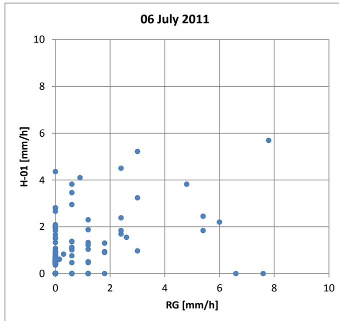
Fig.4 Scatter plot for measured (RG) and satellite derived (H-01) rain rate obtained for all PR-OBS-1 data on the 6<sup>th</sup> of July 2011
