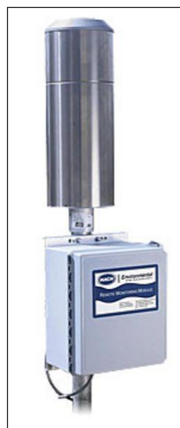
Figure 10 (left): Network of rain gauges in Germany - Figure 11 (right): Pluvio with Remote Monitoring Module
