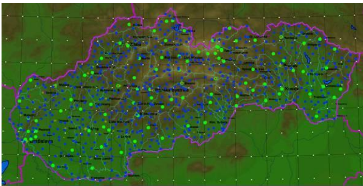
Figure 21 Map of SHMÚ rain gauge stations: green – automatic (98), blue – climatological (586), red - hydrological stations in H-SAF selected test basins (37)
