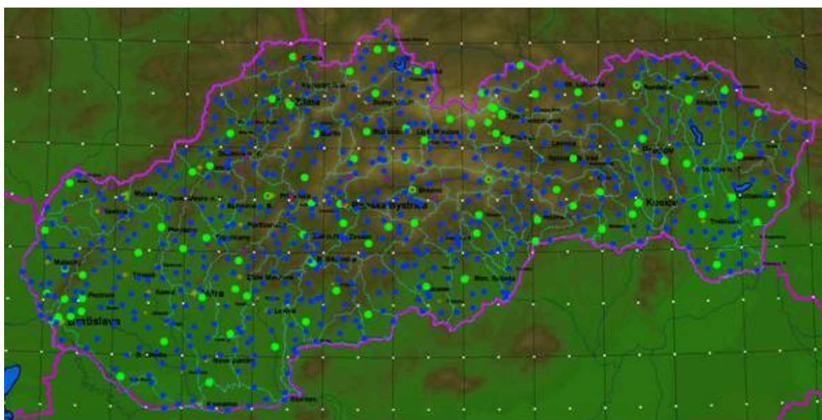
Figure 51: Map of SHMÚ rain gauge stations: green – automatic (98), blue – climatological (586), red - hydrological stations in H SAF selected test basins (37)
