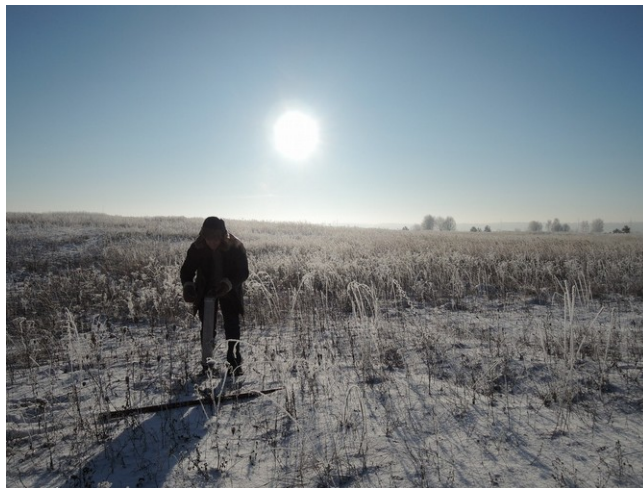
Fig. 13. Snow survey measurements at Vilnius MS. Snow course measurements are done every 10 days in the forest and in the open field. The trails are in vicinity of the station and in most cases fall in the same pixel as meteorological station.
