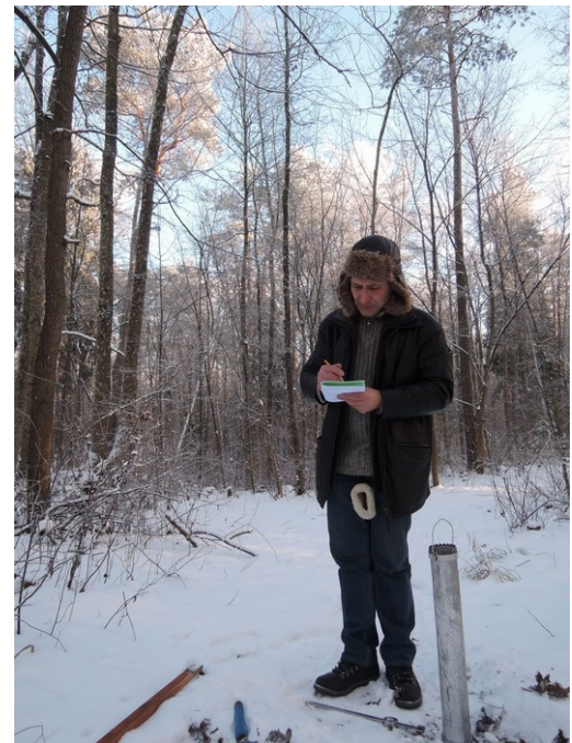
Fig. 13. Snow survey measurements at Vilnius MS. Snow course measurements are done every 10 days in the forest and in the open field. The trails are in vicinity of the station and in most cases fall in the same pixel as meteorological station.
