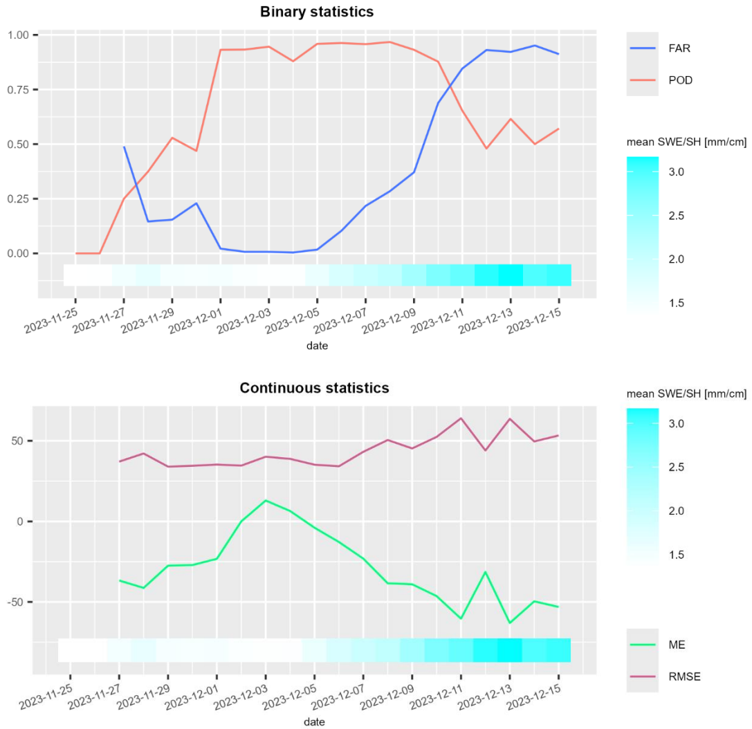
Figure 10: POD [-], FAR [-], ME [mm] and RMSE [mm] over time (25 th November-15 th December 2023) for H65-station-intercomparison (DWD Climate Data Center, 2024; EUMETSAT, 2023) in Germany. Continuous statistics are only computed on the fraction of data where both, H65 and in situ measurements, suggested snow and the snow height measured was between 20 and 100 cm.
